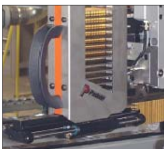
Exchangeable Magazine and Staple reloading Mechanism (feeder)
