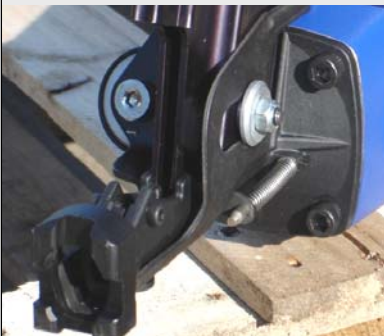
Mechanical safety yoke and special design Contact element reducing drag
