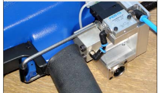
Remote trigger with and without mechanical safety yoke. Nailer is activated with 24 Vdc signal
